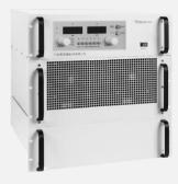
The THP2290 series is a series of closed, programmable, low ripple, high-voltage power supplies that can provide up to 100kV and 25kW power supplies. The THP2290 series is a fast-response power supply and adopts air insulation, so it is lighter and more environmentally friendly than oil cooling.
